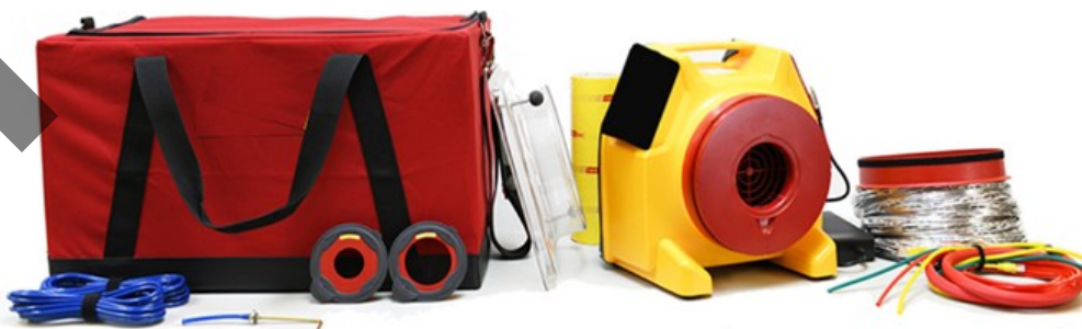
Figure 2-8: Duct leakage test equipment.
