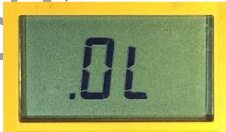
Figure 6-24 Testing at the N.O. terminals on a relay should show “Open Line” without control voltage applied to the relay coil.
