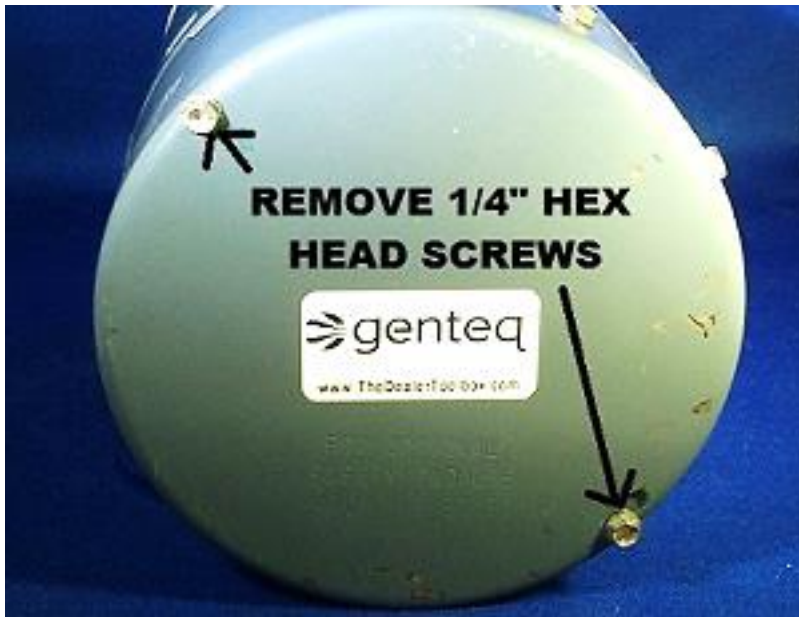
Figure 7-74 Once the power to the equipment has been off for at least five minutes, it is safe to remove the screws and separate the control from the motor case.
