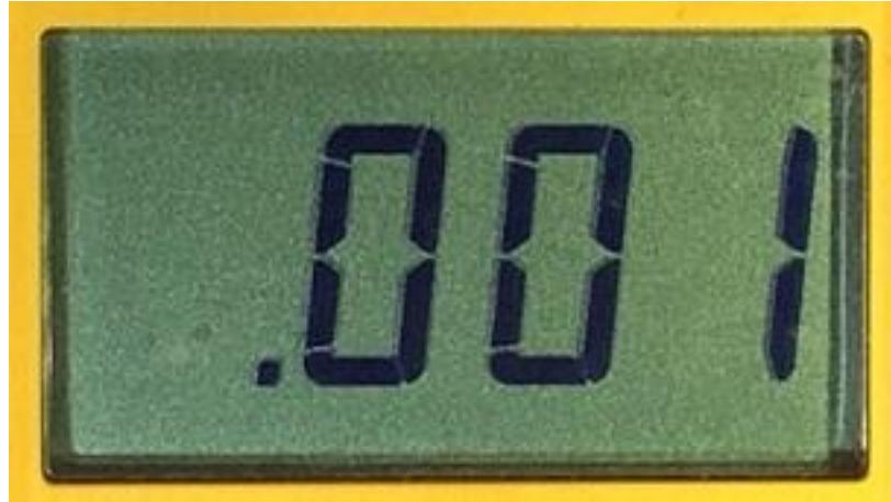
Figure 6-25 If the N.O. relay contacts are in good condition; the meter will display a very low resistance when voltage is applied to the relay coil. In the event that the meter showed 1 Ohm resistance or more, it would indicate that the contacts are corroded, and would cause excessive voltage drop in the circuit.
