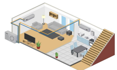
Figure 1-16. Lineset considerations are essential to maintain system efficiency.
