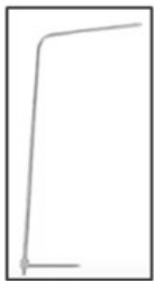
Figure 5-6. A traverse involves determining airflow velocity by taking measurements across different points in the duct using either a pitot tube, hot wire anemometer, or vane anemometer.
