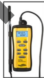
Figure 5-6. A traverse involves determining airflow velocity by taking measurements across different points in the duct using either a pitot tube, hot wire anemometer, or vane anemometer.
