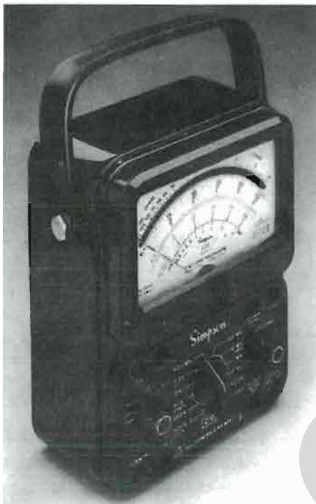
Figure 5-1. A typical analog-type meter used by appliance technicians. Often referred to as a VOM (volt/ohmmeter), it is used for measuring voltage and resistance. (Courtesy of Simpson Electric Co.)
