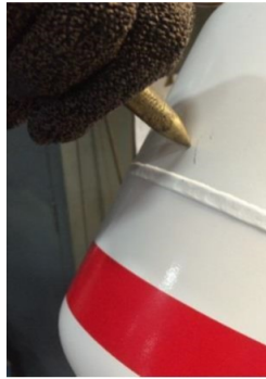
Placement of non-sparking pick for piercing
