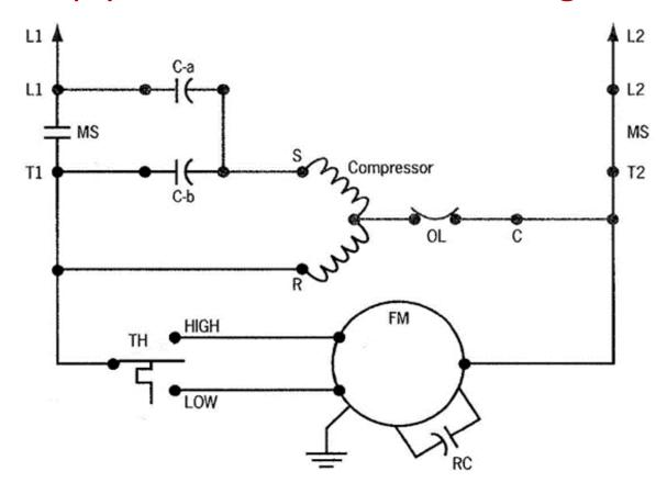
The above diagram shows the circuitry for the compressor and outdoor fan motor of this system.
