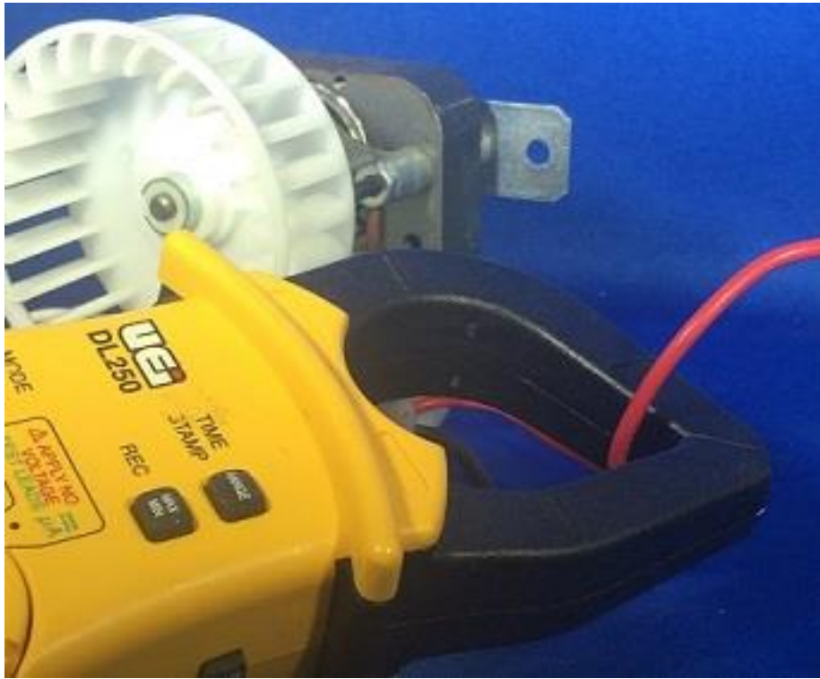
Figure 2-4: A clamp-type meter is used to check the current draw of electrical components in appliances.
