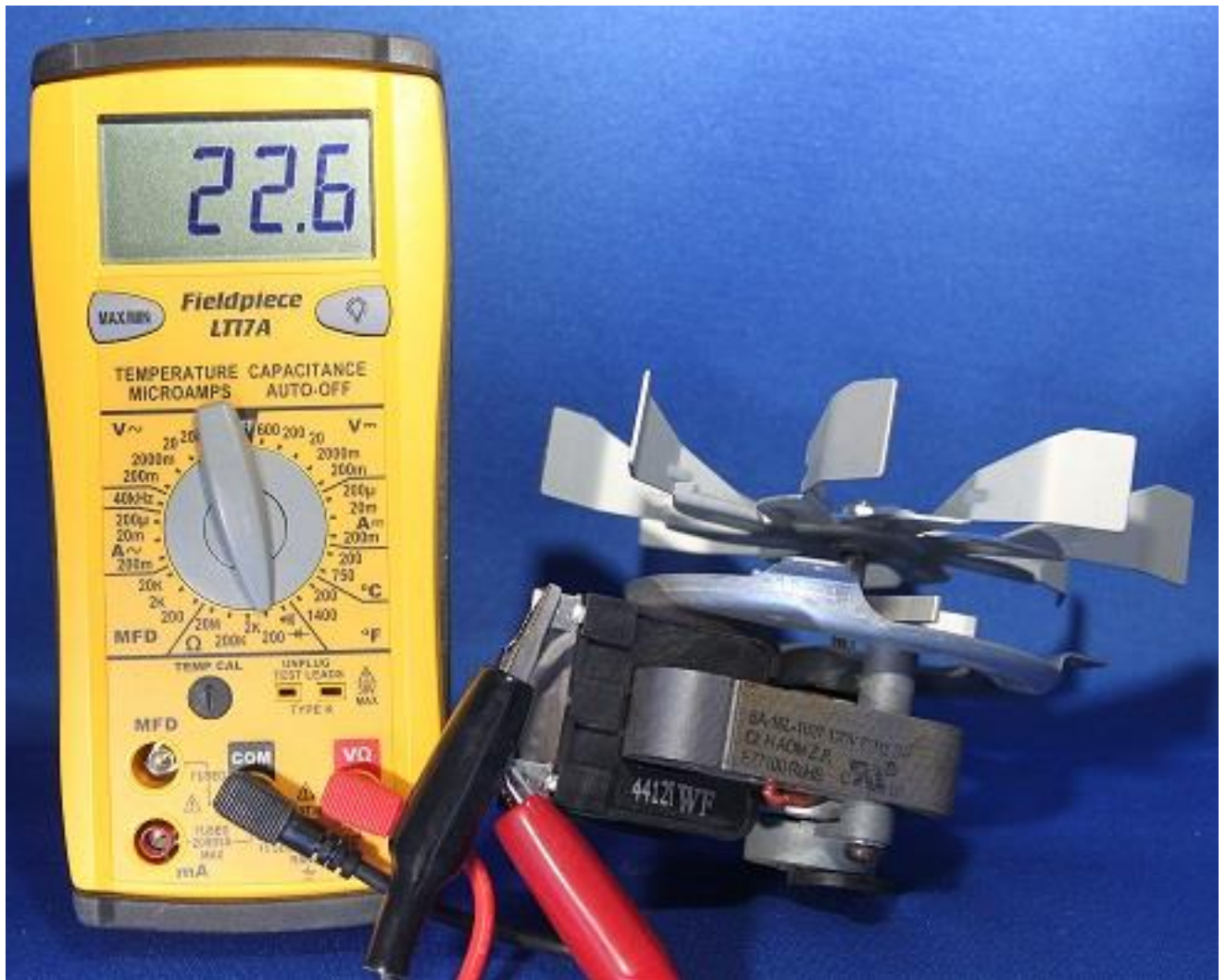
Figure 7-32: In this example, the test equipment is set to a proper range in order to accurately read the resistance of the fan motor, in this case 22.6 Ohms.
