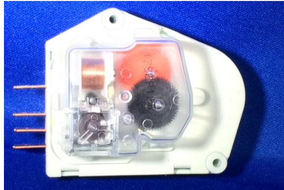
Figure 5-20: One example of a frost-free refrigerator defrost timer in which the motor, switching contacts, and gear assemblies are encased in plastic. The wire harness connections are shown on the left.
