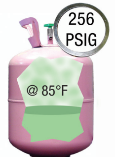
At saturation temperature the refrigerant exists as both a liquid and a vapor simultaneously.
