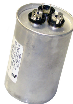
This continuous duty run capacitor is wired in series with the Start Winding in order to create the best magnetic hold possible on the motor rotor.
