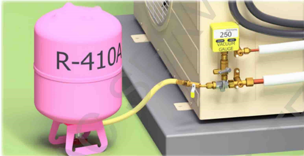
Figure 7-28: Step 10-B of the Vacuum Procedure with a Bottle
