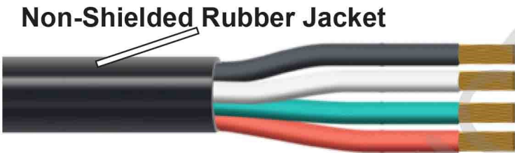
Figure 12-9: Non-Shielded Communication Wiring
